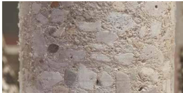
**Fig. 2:** This core sample shows how integrally the first lift and second lifts bond. The frayed fibers visible on the cut surfaces of the core provide the only obvious evidence that the slab was placed in two lifts (Photo courtesy of Joe Nasvik)
